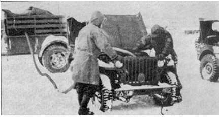
Soldiers of Task Force Frost use a "slave kit" mounted on a one-ton trailer to heat a jeep engine during tests of cold-weather starting devices at Camp McCoy, WI, in 1946.
